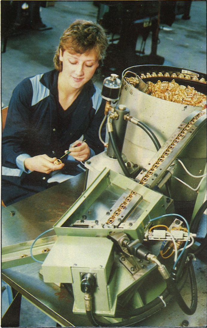
Mrs Anne Beale marking domes of lampholders with earthing symbols. At the same time, the dome is pierced to take the earth terminal block.
