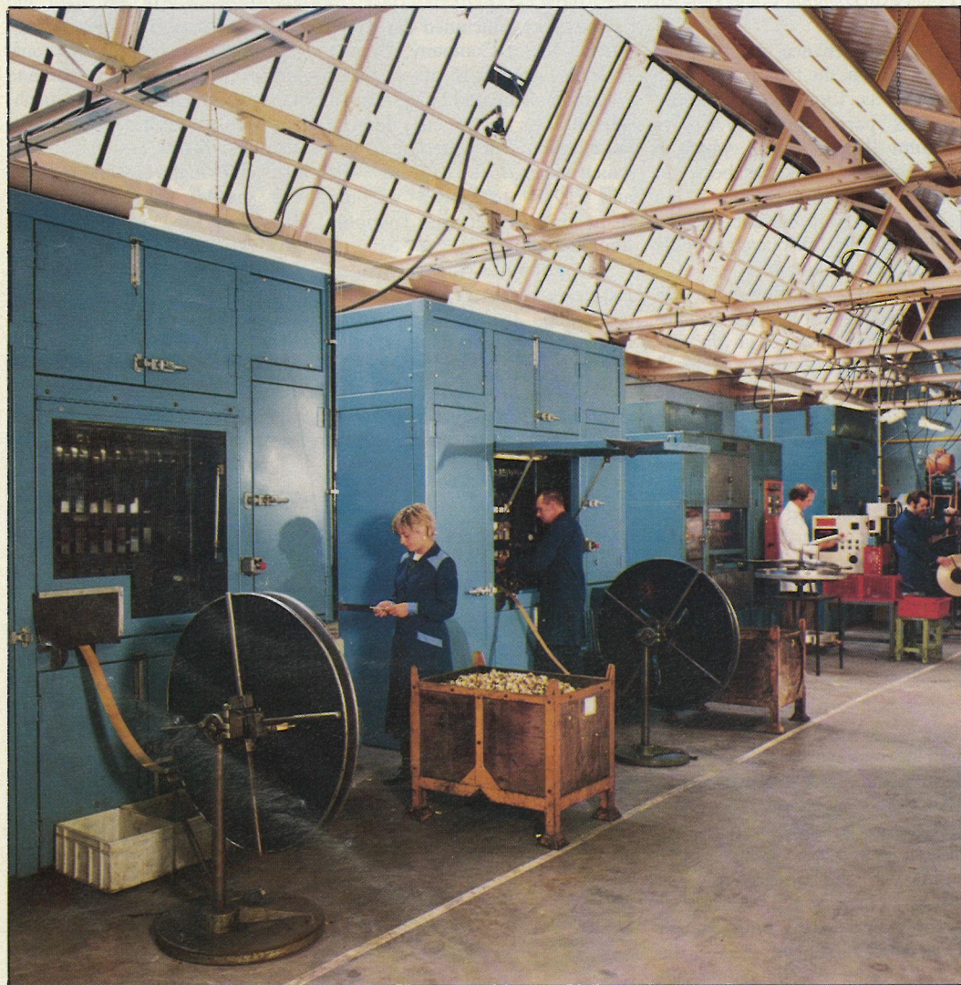
Lampholder bodies and domes are produced by automated methods.
