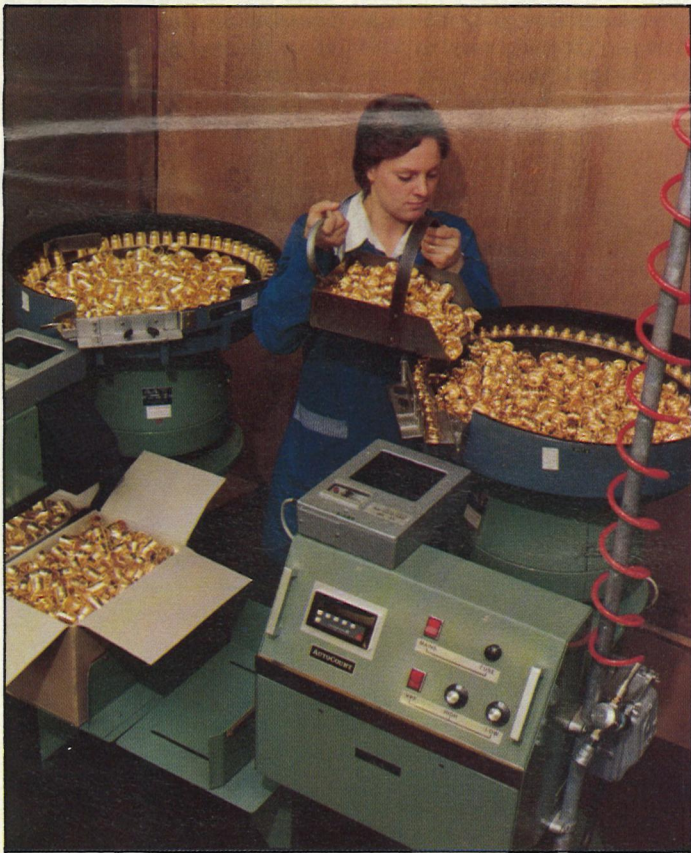
Mrs Glennis Taylor loading the bowl feeder of the unit which count checks the brass domes used in IMI Reeves lampholders.
