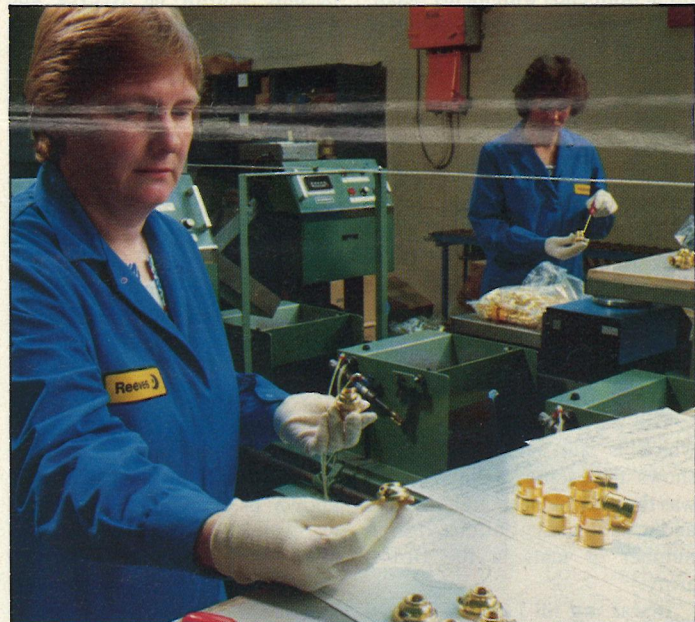
Quality control and inspection of lampholder components: foreground: Christina Cheshire; background: Karen McGuire.
